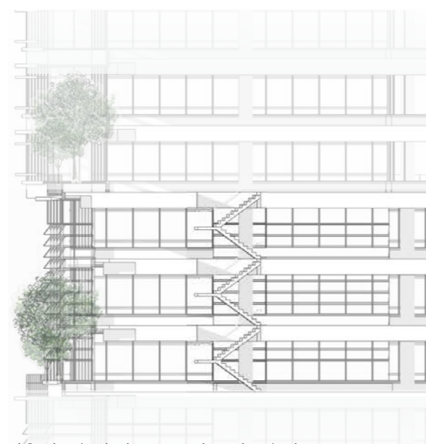
/ Section showing interconnecting stair and atrium spaces
